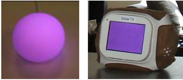
Figure 3: The orb and Chumby devices displaying a purple color (more than one friend is watching TV).
